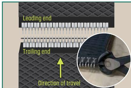
Chamfer corners of the belt's trailing end.
