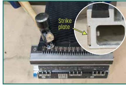
Flatten the rivets on the reinforced strike plate. Do not strike or damage the loop area of the fasteners! *(Tip: use the peen on a ball peen hammer to flatten rivets).*
