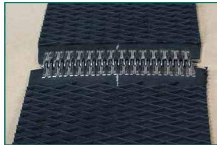
To join ends, connect the fasteners with the correct offset so that the belt edges line up.
