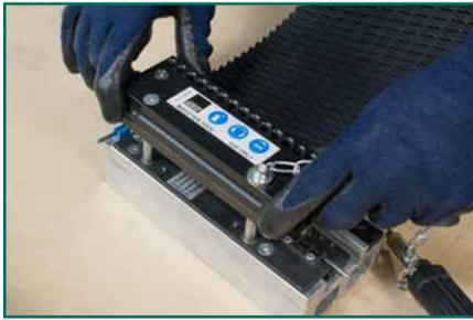
Mount the guide block so that all the rivets are inserted into the holes of the block. Each hole will accommodate two rivets.
