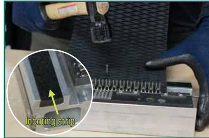
Secure the belt to the locating strip with staples or small nails.
