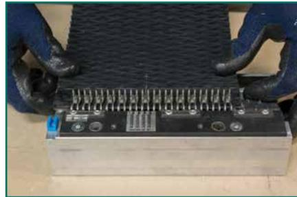
Insert belt into the fastener strip and against the belt stops. Align the belt's center line with the appropriate selection on the sticker. *(Tip: the number of fasteners on the selection sticker refers to the segment count. Example: a seven inch wide belt requires a fastener strip with 14 segments).*
