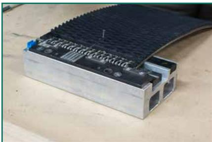
Remove the guide block after setting all the rivets, remove holding pin, and then remove the splice from the tool. *(Tip: if the guide block is difficult to remove, use a flat head screwdriver to leverage the block up for easier removal).*
