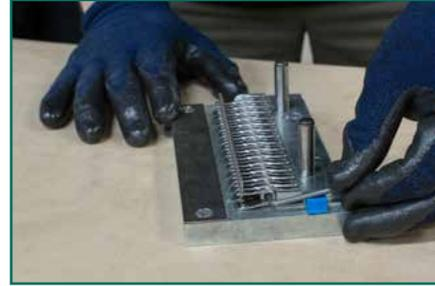
Insert holding pin to secure the fastener strip.
