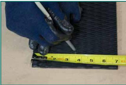
Mark the belt ends for fastener positioning. Place a mark 1.5mm (1/16") offset from the centerline on both belt ends toward the same side of the belt.
