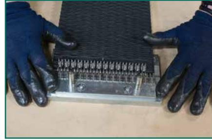
Insert belt into the fastener strip and against the belt stops. Align the center of the fastener strip with the offset mark on the belt end. *(Tip: pre-mark the tool's fastener holder for the center of frequently used widths of fastener strips).*
