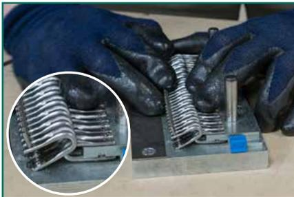
Insert fastener strip into the tool. Make sure the fastener strip is properly placed with the pins resting in the recesses of the fastener. *(Tip: load the back of the plate first, then swivel the loops down and into place).*
