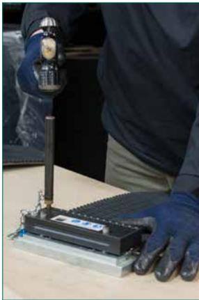
Use a 1/2 pound hammer to set the rivets (do NOT use a pneumatic hammer). Follow the sequence shown for the first three fastener segments. Continue to set the remaining rivets in any sequence. *(Tip: be sure all rivets have been set prior to removing the splice from the tool).*
