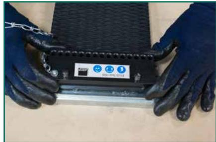
Mount the guide block so that all the rivets are inserted into the holes of the block. Each hole will accommodate two rivets. *(Tip: be careful not to jostle the belt out of position).*
