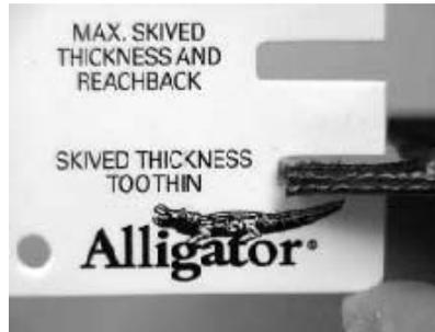
**How far back onto the belt should you remove the impression top?** The skived portion of the belt must fit entirely into the gauge. If the gauge does not fit entirely on the skived portion of the belt you must remove more of the impression top.
