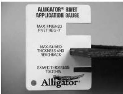
**Can you remove too much impression top?** Yes! A belt can be skived too thin. A belt that is too thin may not allow the rivets and fastener strip to be compressed enough. If there is a gap between the belting and the gauge, the belt end must be cut off and the belt must be skived again. It is also critical to not expose the fabric of the top ply of the belt.
