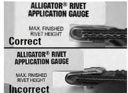
**How do you know when the fastener is installed correctly?** Installing Alligator® Rivet requires striking the fastener strip several times with a 1 lb. hammer. The gauge should easily slide onto your fastener strip after installing. If the gauge does not slide over each plate the fastener strip needs to be placed in the tool and struck several more times to ensure proper compression.
