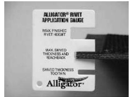
**How much impression top do I remove?** The gauge will tell you when you have removed enough impression top to allow proper installation of the Alligator Rivet fastener. When the gauge can be placed on the belt and can slide across the width without encountering resistance the belt has been properly skived. If the gauge cannot be inserted onto the belt then additional impression top must be removed.
